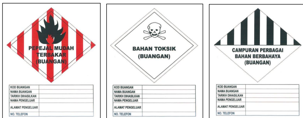
Figure 9.6.2: Example of Proper Labeling of Scheduled Waste
